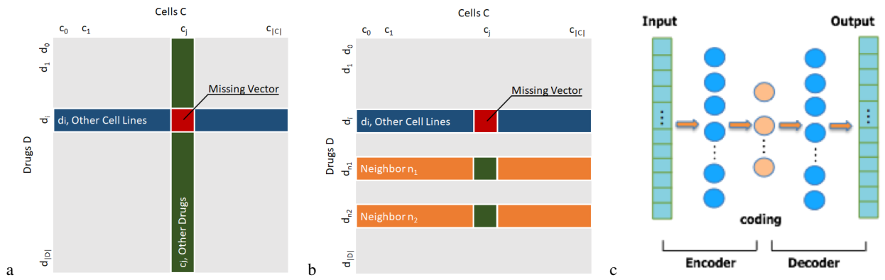
Fig. 1. Fig. 1. Methods overview. a) In tissue-agnostic imputation, the median of the expression profiles (vectors) for drug d_i on cells other than c_j (in blue) is used to predict the unknown expression profile for drug d_i on cell c_j . The two-way average is the average of two sets of expression profiles: the median of the expression profiles for drug d_i on cells other than c_j (in blue) and the median of the expression profiles for drugs other than d_i on cell c_j (in green). b) In the neighborhood approach to collaborative filtering imputation, neighbors are drugs whose expression profiles on cells other than c_j (in orange) are most similar to d_i 's profile on cells other than c_j (in blue). In this example with x = 2 neighbors, the expression profile for cell c_j on neighbor drugs d_{n_1} and d_{n_2} , shown in green, are used to impute the profile for drug d_i on cell c_j . c) In the autoencoder approach, a lower-dimensional coding representation of cell and drug specific expression profiles are learned through an encoder and then decoded back to reconstruct the original data or to predict the expression profiles of missing cell and drug combinations.
